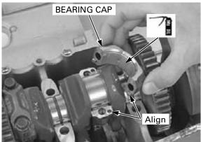
The connecting rod bolts cannot be reused. Once the connecting rod bolts have been loosened, replace them with new ones.
