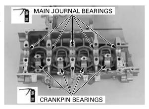
Apply molybdenum oil solution to each thrust surface of the crankshaft as shown.
