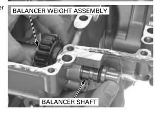
Pull the balancer shaft out and remove the balancer weight assembly from the lower crankcase.
