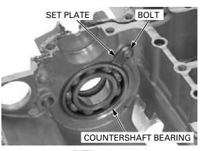
Remove the countershaft bearing from the lower crankcase using the special tool.
