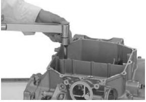
Tighten the 8 mm bolt to the specified torque.
