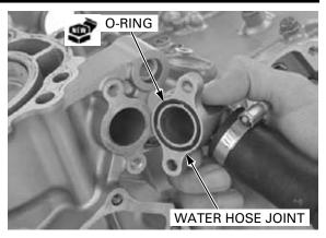
Install the water hose joint to the crankcase, then tighten the two bolts securely.
