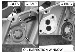
Remove the bolts, clamp and oil inspection window. Remove the O-ring from the oil inspection window.
