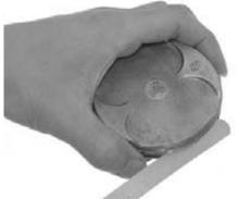
Push the rings into the cylinder with the piston head to be sure they are squarely in the cylinder.
