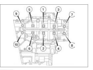
Further tighten the crankcase 9 mm bolts (main journal bolts) 150 degrees.
