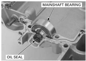
Remove the mainshaft bearing and clutch lifter rod oil seal from the upper crankcase.
