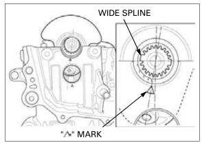
5. Carefully place the lower crankcase onto the upper crankcase.
