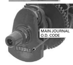
Cross reference the main journal and bearing support codes to determine the replacement bearing . color code.
