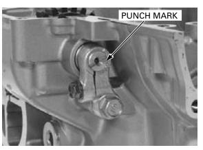
2. Remove the sealing bolt and sealing washer from the lower crankcase.
