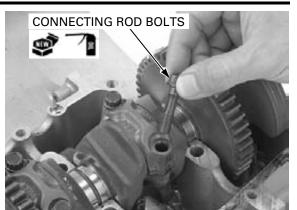
Tighten the connecting rod bearing cap bolts with a Plastic Region Tightening Method.
