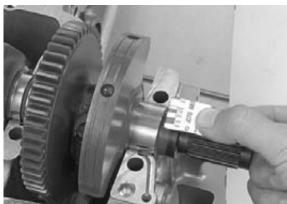
on the left side of upper crankcase are codes for the bearing support I.D. from left to right.
