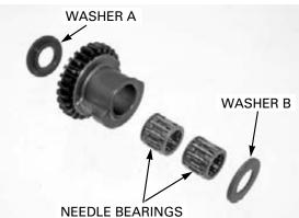
Remove the balancer gear assembly from the balancer weight.
