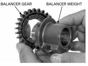
Remove the damper rubbers from the balancer gear.
