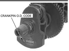
Cross-reference the connecting rod and crankpin codes to determine the replacement bearing color.
