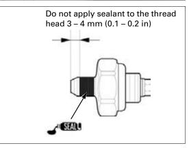
Apply a sealant (Three Bond 1207B) to the oil pressure switch threads as shown.
