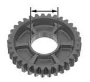
Measure the O.D. of each gear bushing.
