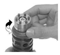
Inspect the shift drum guide grooves for abnormal wear or damage.
